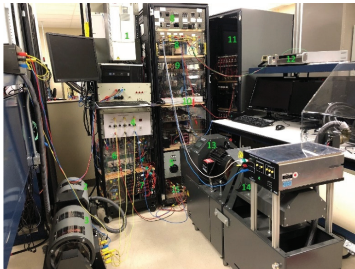
Figure 5. Hardware prototype of hybrid wind-PV-diesel off-grid system.
