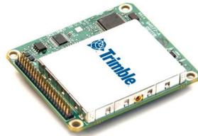
**Figure 3.** Trimble APX-15 Unmanned Aerial Vehicle (UAV) single board Global Navigation Satellite System (GNSS)-inertial solution.
