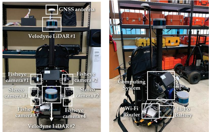
Figure 1. Backpack-based Multi-Beam Light Detection and Ranging (LiDAR) (MBL) sensor system.
