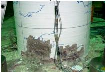
loading specimens (RH-NS-T). (**a**) Spalling of the concrete on the outside face of the rete cover concrete on the outside face of the top  $(8\Delta_y)$ ; (**c**) Failure of the concrete cover  $(8\Delta_y)$ .
