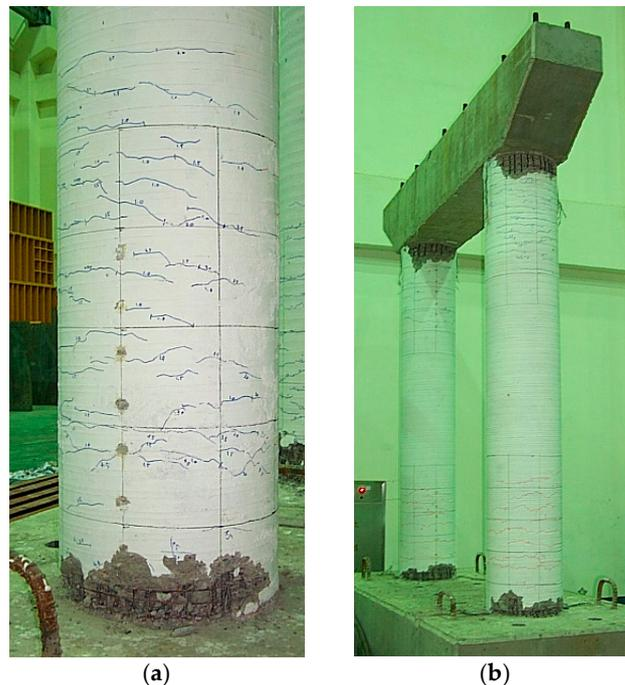
**Figure 10.** Failure of a longitudinal loading specimen and a transverse loading specimen. (a) Failure at the bottom of the column of the RH-NS-L specimen; (b) Failure at the top and bottom of the column of the RH-NS-T specimen.
