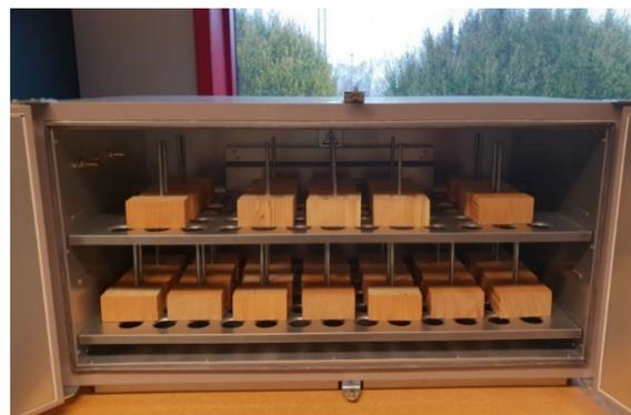
**Figure 2.** Preparation of specimens under controlled atmosphere.
