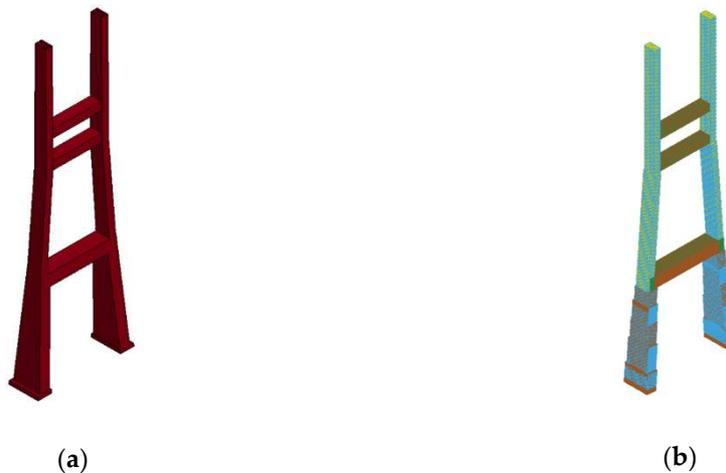
Figure 5. Pylon model: (a) concrete part and (b) rebar.
