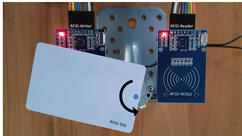
Figure 3. RFID data collection.
