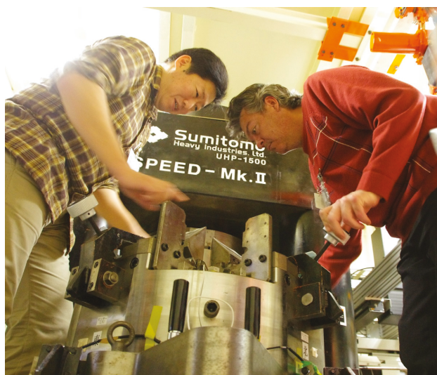
Figure 5. Ken-ichi Funakoshi and Mark Reid loading the pressure cell and sample into the 15-MN press SPEED-Mk.II at SPring-8 beamline BL04B1.
