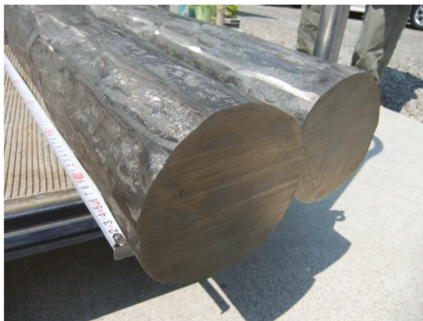
Figure 2. Photograph of the forged ingot that is approximately 100 mm in diameter, which was mechanically thinned from the VAR-fabricated TiZr ingot that was 240 mm in diameter.
