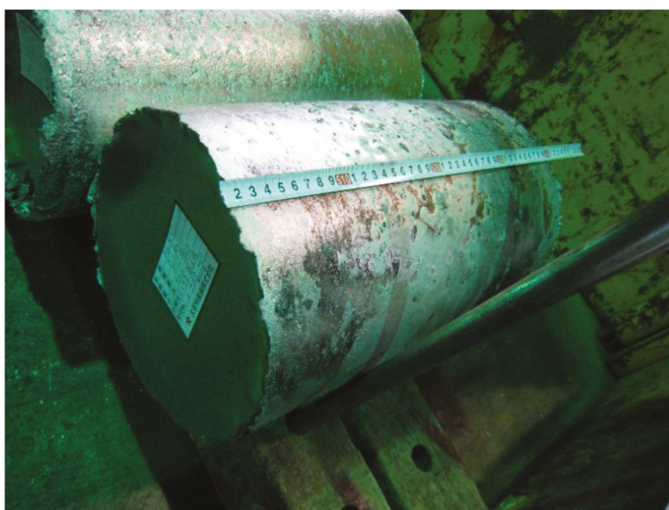
Figure 1. Photograph of the VAR-fabricated TiZr ingot, which was 240 mm in diameter, 384 mm in length, and 85.4 kg in weight.
