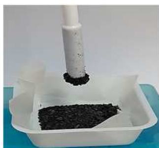
Figure 3. Dry grinded ZVI@ORMOSIL powder on a magnetic bar.
