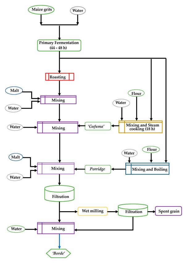
Figure 1. Borde processing flow chart [29].
