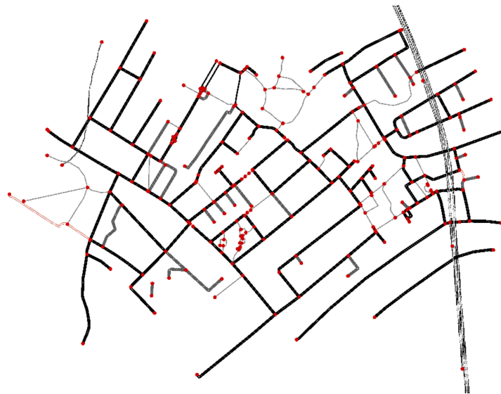
Figure 1. Representation of a road network as a graph of vertices and edges.
