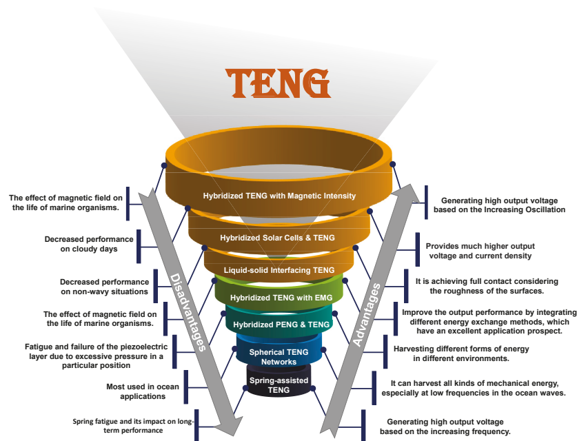
Figure 13. Advantages and disadvantages of different TENG structures.
