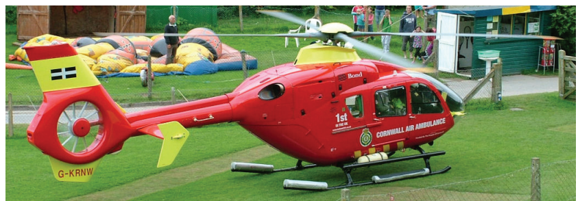
Figure 1. Eurocopter EC 135, with a fantail assembly tail rotor (reproduced from https://en.wikipedia.org/wiki/Tail_rotor accessed on 21 April 2021).
