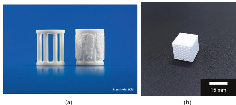
**Figure 2.** Overview samples vs. Curasan control: (a) VPP-manufactured column support structure (left) and hybrid with Freeze Foam enclosing the VPP support (same figure, right); (b) Curasan control.
