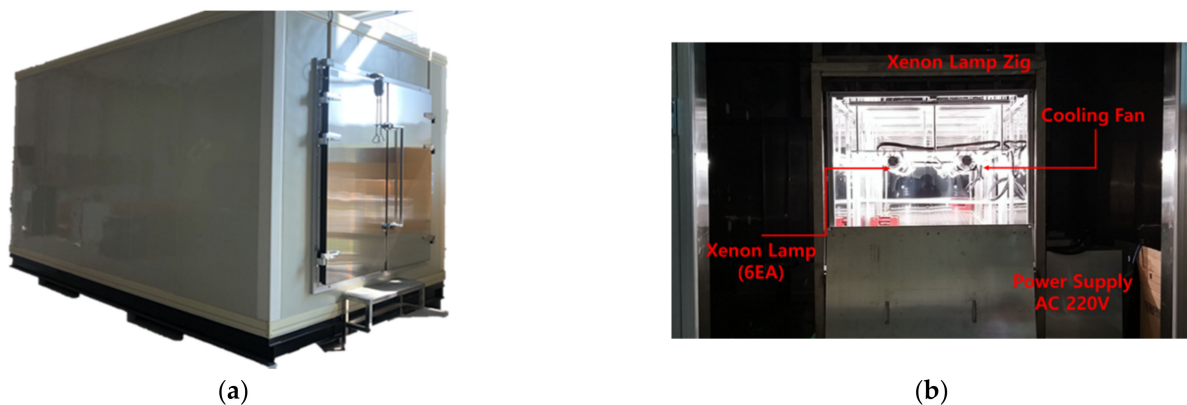
Figure 1. Photographs of the (a) exterior and (b) the interior of the PV panel experimental chamber.
