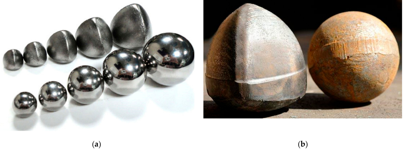
Figure 1. Grinding media charges: (a) Relo M-1 vs. balls (b) Relo M-2 vs. ball.
