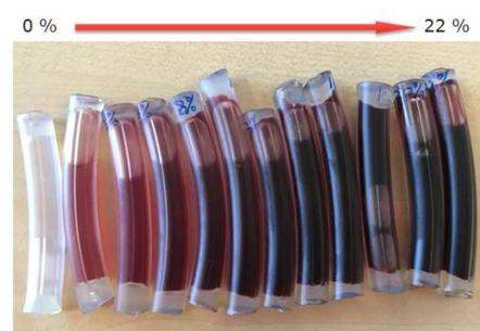
**Figure 9.** Test specimen samples. Tube segments were filled with diluted blood and sealed with hot glue. In order to test the effect of bubbles, a small fraction of air was left inside. This also prevented direct contact between the hot glue and test liquid. Samples were produced for blood concentration between 0% and 22% in increments of 2%. *Hb* concentration was measured using a hemoglobin analyzer.
