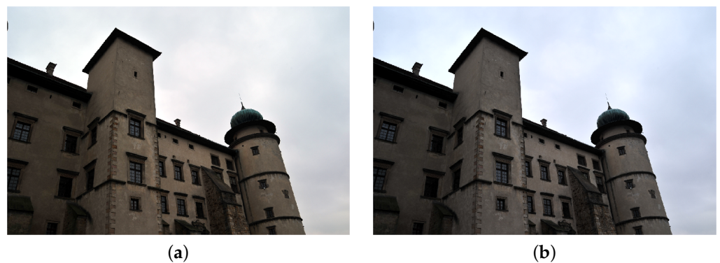
Figure 3. Image transformed with the use of histogram stretching in RGB (a) and L^*a^*b^* space (b).
