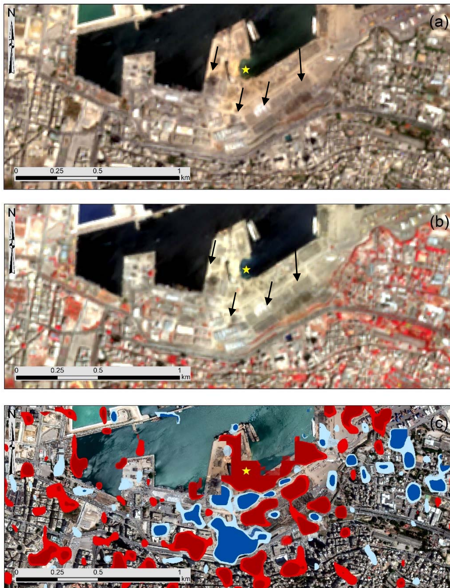
Figure 9. (a) Sentinel-2 optical image taken over the area of interest on the 8th of August 2020 (RGB composite). (b) The NIR-R-G pseudo color composite of the same image and (c) the change detection results from the Sentinel-1 image analysis. Black arrows indicate destroyed areas from image interpretation of the Sentinel-2 image, while yellow arrows indicate the non-detectable destroyed areas from this analysis. The location of the blast site is shown with the yellow star.
