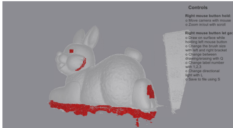
Figure 10. View from the annotation tool used for creating the roughness versus noise ground truth for each of the meshes. The vertices painted red are set as reconstruction noise.
