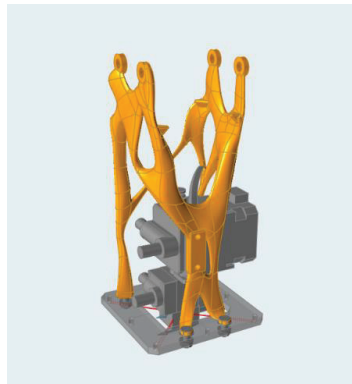
Figure 9. Remodeled component with PolyNurbs.
