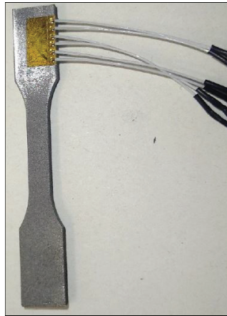
Figure 2. Strain gage method in hole drilling for measurement of residual stresses.
