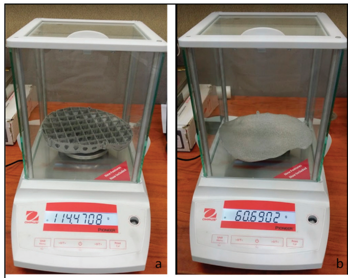
Figure 11. Weighing scale reading of cranial implants (a) with supports and (b) without supports.
