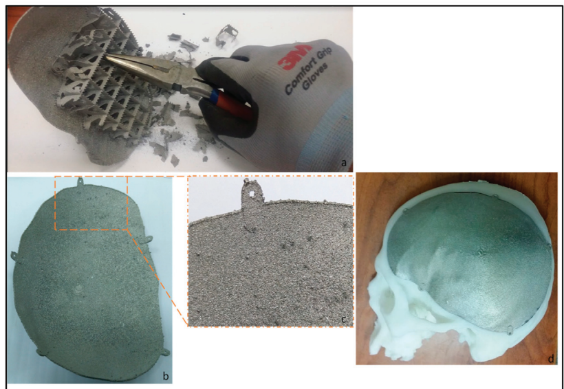
Figure 7. (a) Removal of support structures using pliers, (b,c) illustration of protrusion onto the surface of the cranial implant after the removal of supports, and (d) implant fitted onto the polymer skull model.
