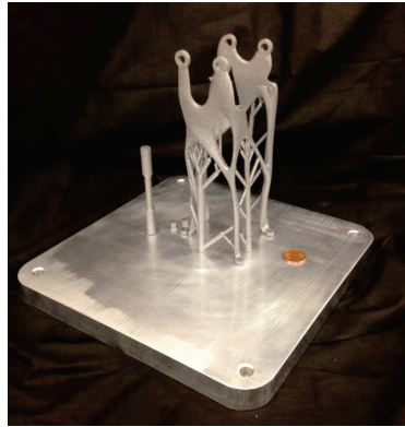
Figure 11. Real component made by SLM (small series).
