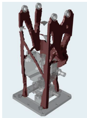
Figure 8. Material density distribution after topology optimization.
