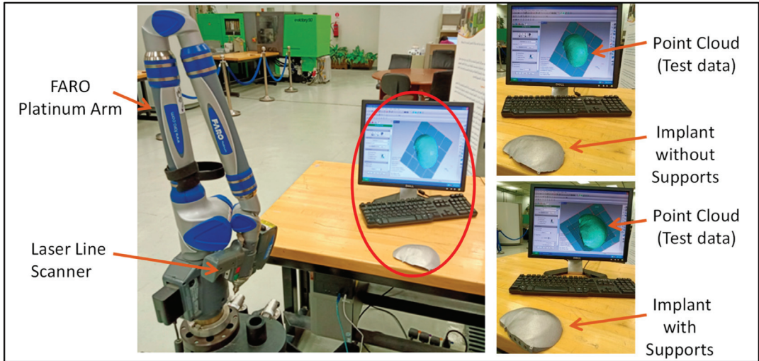
Figure 13. Set up to capture point cloud data for the fabricated models.
