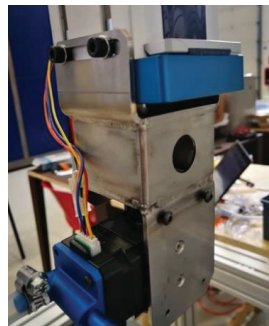
Figure 5. Fused Deposition Modeling (FDM) head of PEEK extrusion machine.
