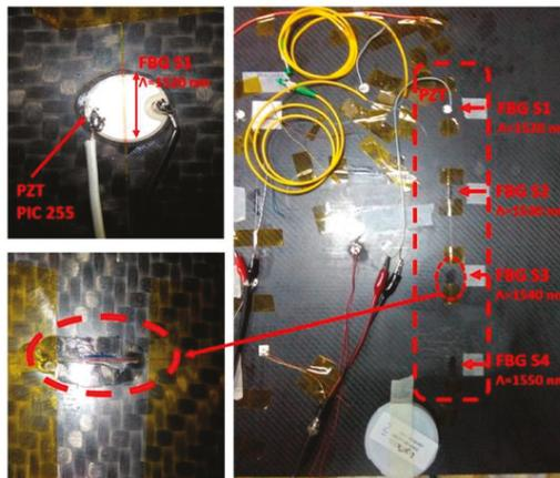
**Figure 6.** Composite panels setup and differential strain distribution [48].
