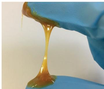
**Figure 1.** Thread formation during physical separation of a grease.
