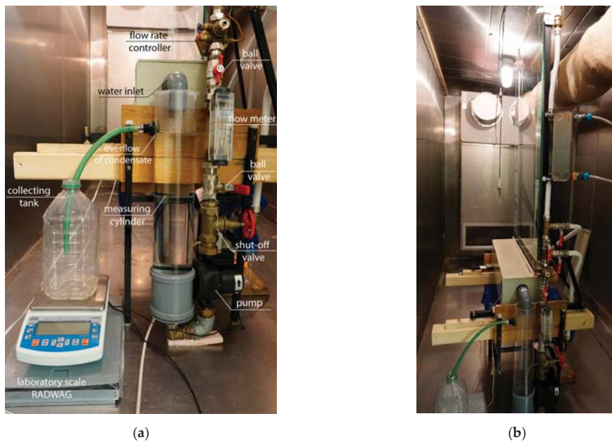
Figure 8. The measuring system for dehumidification performance: (a) Detailed view of the system; (b) Overall view of the system and the water wall located in the climate chamber.
