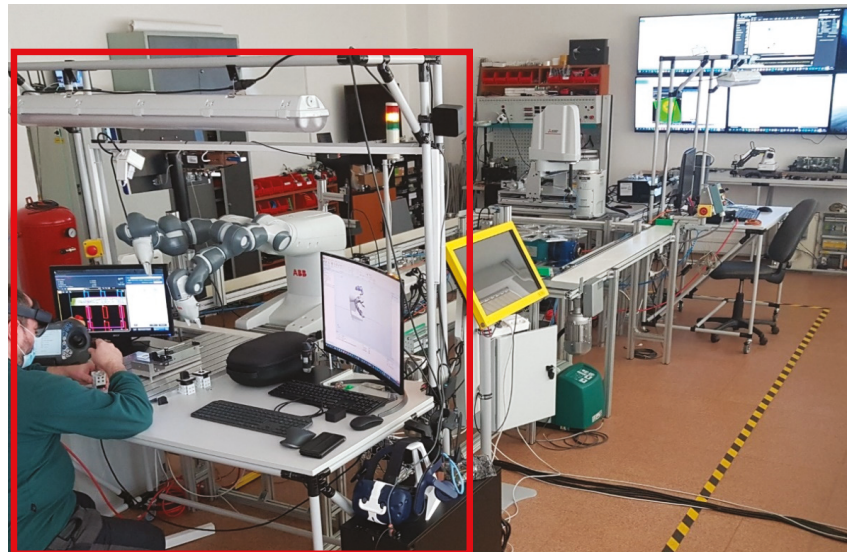
Figure 3. The experimental SMART manufacturing system; red frame: the workplace with an assisted assembly work cell with collaborative robot ABB Yumi and Microsoft Hololens 2 mixed reality device.
