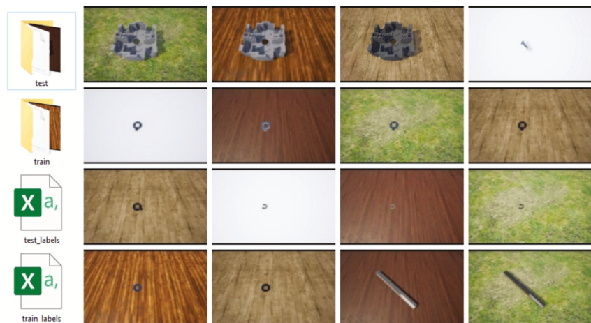
Figure 12. An example of the autogenerated training/ tests set with XML bounding box annotation.
