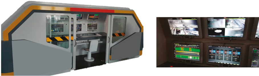
Figure 2. Cabin for monitoring the automatic operation of the MIKRUS system from the surface [8].
