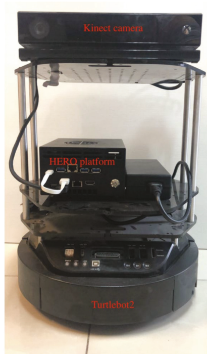
Figure 1. The processing platform.
