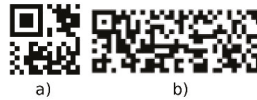
Figure 2. Other types of a QR Code: (a) Micro QR code, (b) iQR code.
