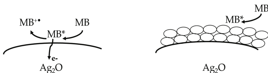
Figure 7. Possible mechanism of MB bleaching by \text{Ag}_2\text{O} and \text{Ag}_2\text{O} -containing mixtures and composites under visible light illumination.
