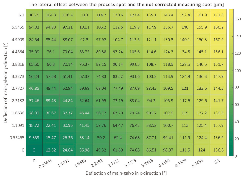
Figure 6. Lateral offset between the process spot and the not corrected measuring spot in dependency of the deflection of the two main-galvanometers.
