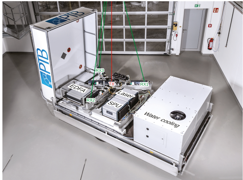
Figure 3. The PTB high-resolution bistatic lidar is mounted on a custom-designed trailer with a hinged cover (opened here), under which the optical set-up and the signal processing unit (SPU) are located.
