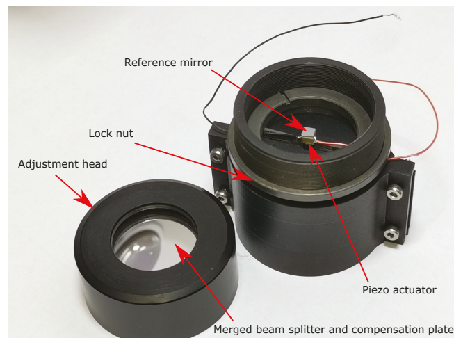
Figure 2. Photograph of the custom-built MA with demounted adjustment head for better view of the used piezo actuator.
