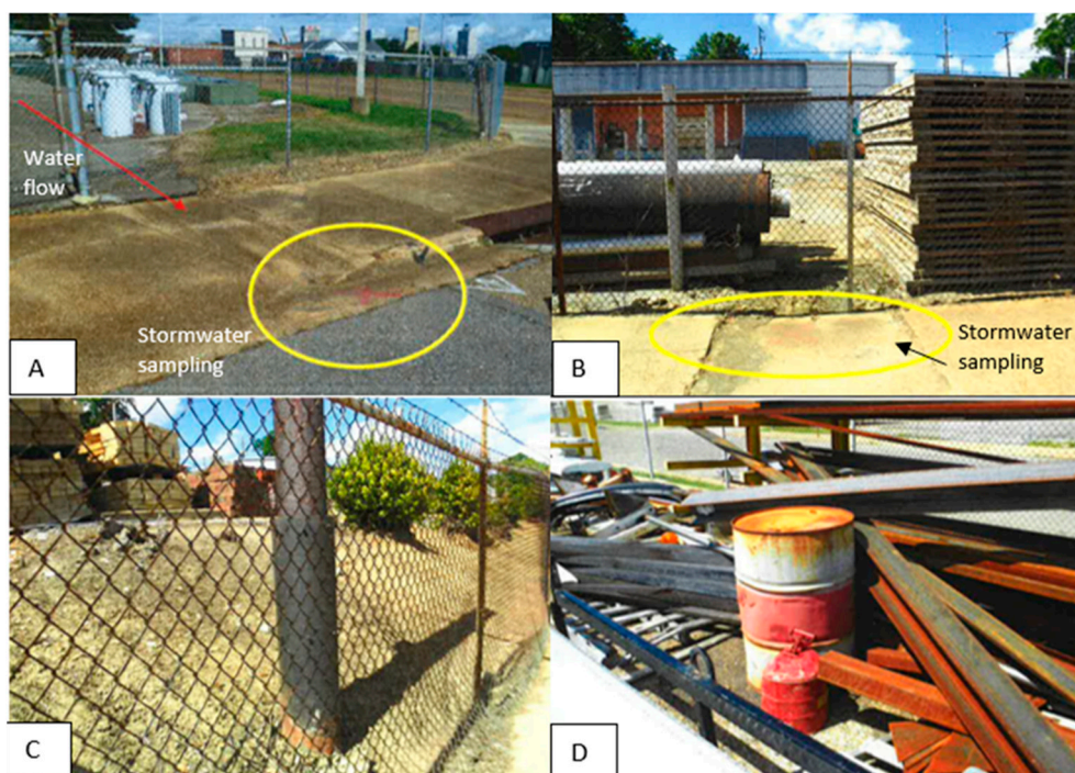
Figure 2. Various sources contributing to storm runoff contamination at (A) Facility A1, (B,C) Facility A3, and (D) Facility A6 (Photos obtained from State Regulatory Agency’s inspection reports in 2015).
