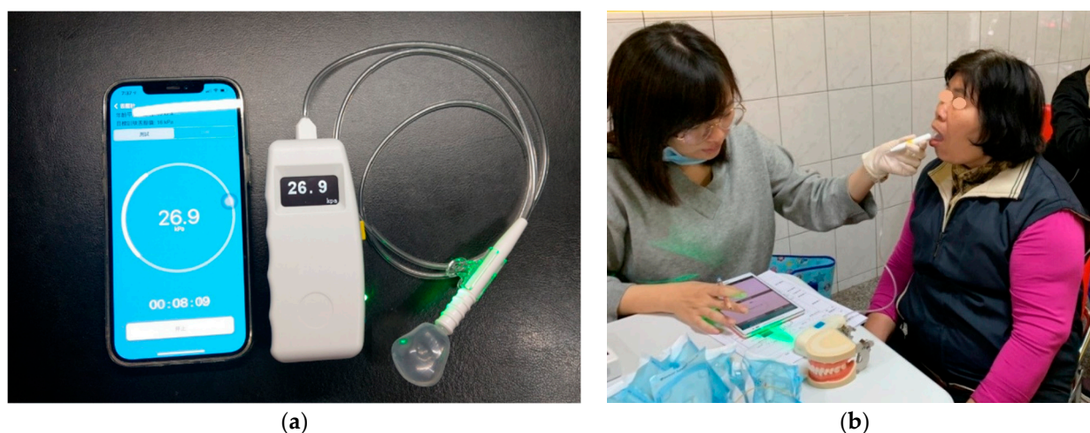
Figure 1. (a) A tongue pressure measurement device with wireless mobile application control function and a disposable oral positioning mouthpiece. (b) The tongue pressure device and its usage in the measurement of tongue pressure.
