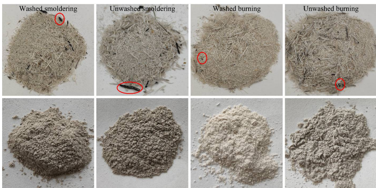
Figure 4. Photos of four types of rice husk ash (circles show black particles in ash).
