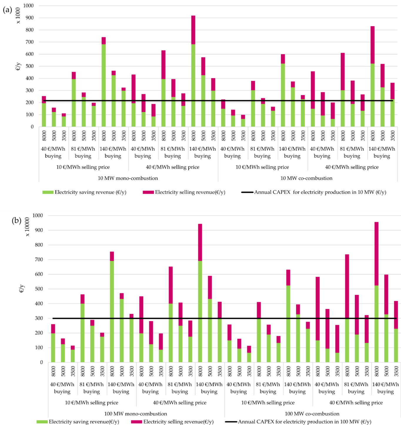
Figure 4. Total annual costs versus economic benefits of electricity production in the (a) 10 MW and (b) 100 MW mono-/co-combustion scenarios, respectively and for different electricity buying prices (40, 81, 140 €/MWh) and selling prices (10, 40, 60 €/MWh).
