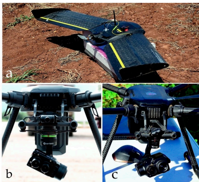
Figure 9. (a) The fixed-wing Q100 Datahawk; (b) the multispectral Sentera camera; (c) the thermal infrared camera Zenmuse XT2.
