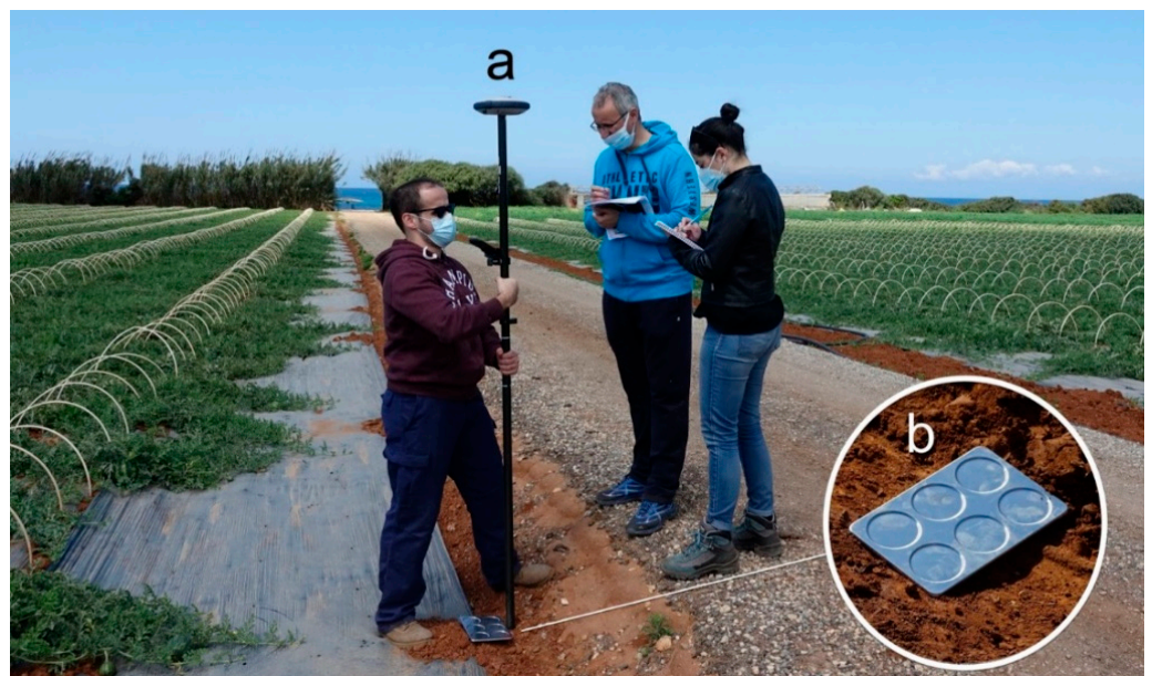
Figure 11. (a) The RTK GNSS that was used for the collection of the GCPs; (b) the rectangular aluminum plates that were used as ground control points on the field.
