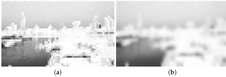
Figure 6. (a) Backlight without Improved Blur Mask Approach; and (b) backlight with Improved Blur Mask Approach.
