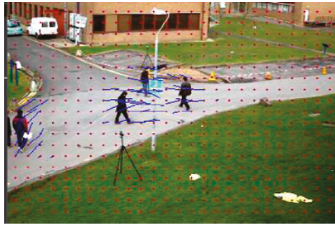
Figure 2. Motion detection through optical flow.
