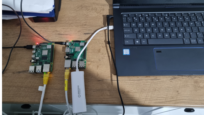
Figure 4. Experiment setup with IoT devices/nodes (RPi 4B), IoT gateway (RPi 3B+), deployment controller (laptop).
