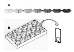
**Figure 2.** Schematic representation of the two most widely used non-forced multi-compartmented exposure systems in avoidance experiments: (**A**): linear system representing a contamination gradient indicated by the scale of grey and (**B**): HeMHAS (Heterogeneous Multi-Habitat Assays System) with the gate used to open or close the connections between compartments in all directions.
