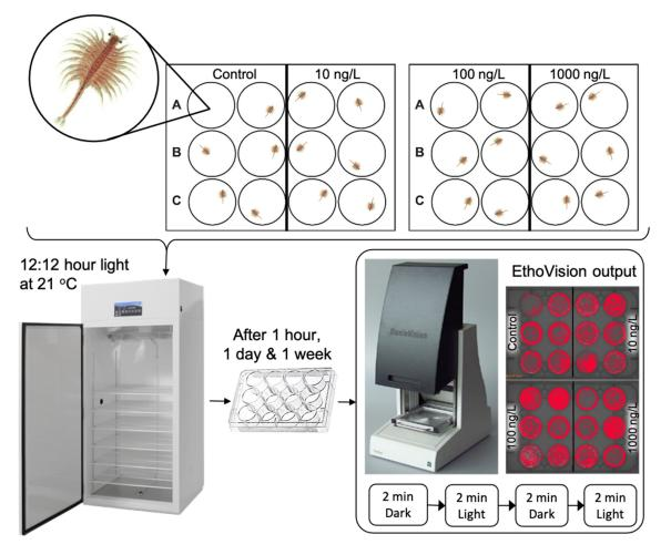
**Figure 2.** Experimental design for *A. franciscana* exposure and behavioural analysis. The 12-well plates were loaded in duplicate to provide 12 replicates per treatment. The procedure was repeated for each of the four compounds.
