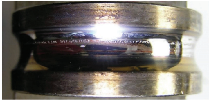
Figure 4. Pitting on a ball bearing inner ring after its test run, reprinted with permission from ref. [20].
