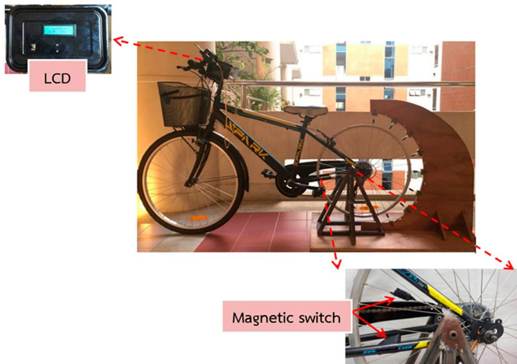
Figure 5. The speed measuring devices mounted on energy harvesting exercise bicycle.
