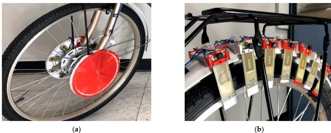
**Figure 7.** The actual installation of piezoelectric modules on a bicycle: (a) Piezoelectric modules installation distance at front wheel; (b) Piezoelectric modules installation distance at rear wheel fenders.
