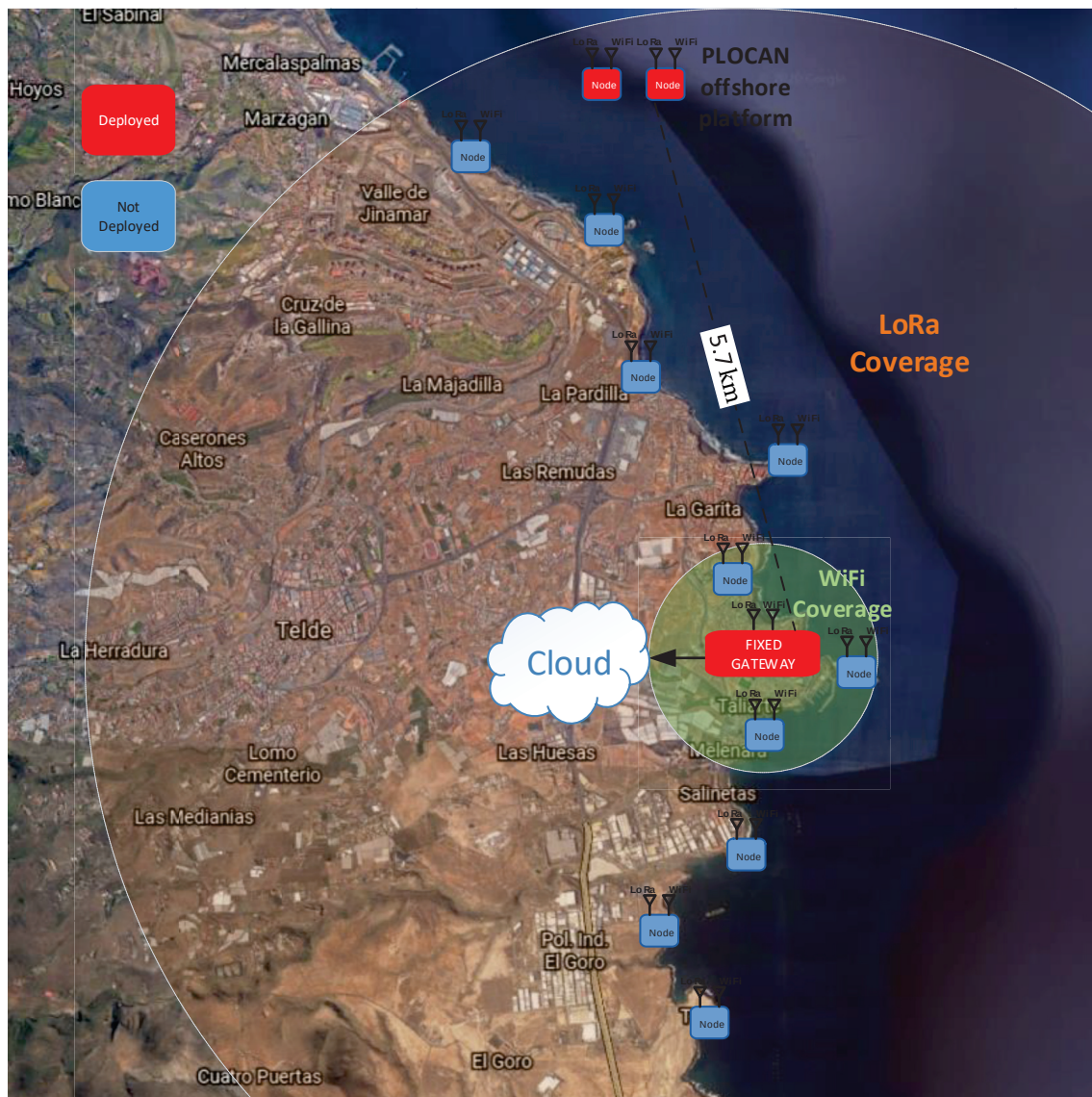
Figure 2. Proposed flexible Fog Computing architecture.
