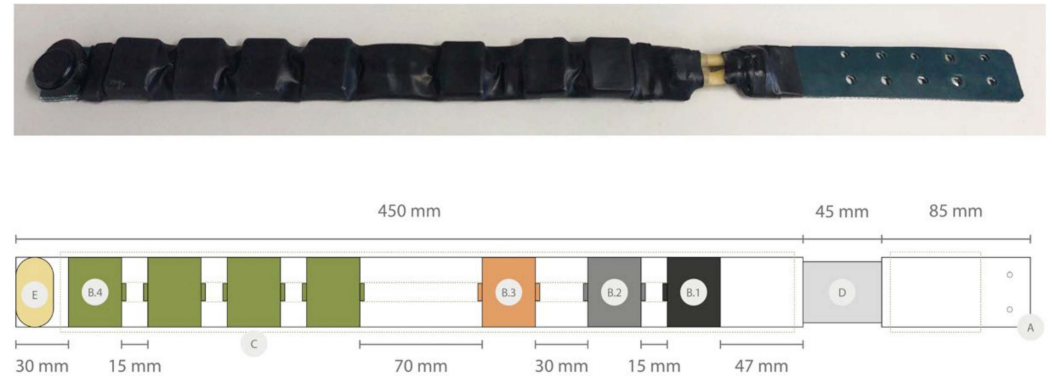
Figure 4. Bounded distribution of the elements of the collar (A Strap; B.1 GPS module; B.2 Communications module; B.3 Sensors module; B.4 Battery modules; C Coating; D Drop-Off; E Closure).
