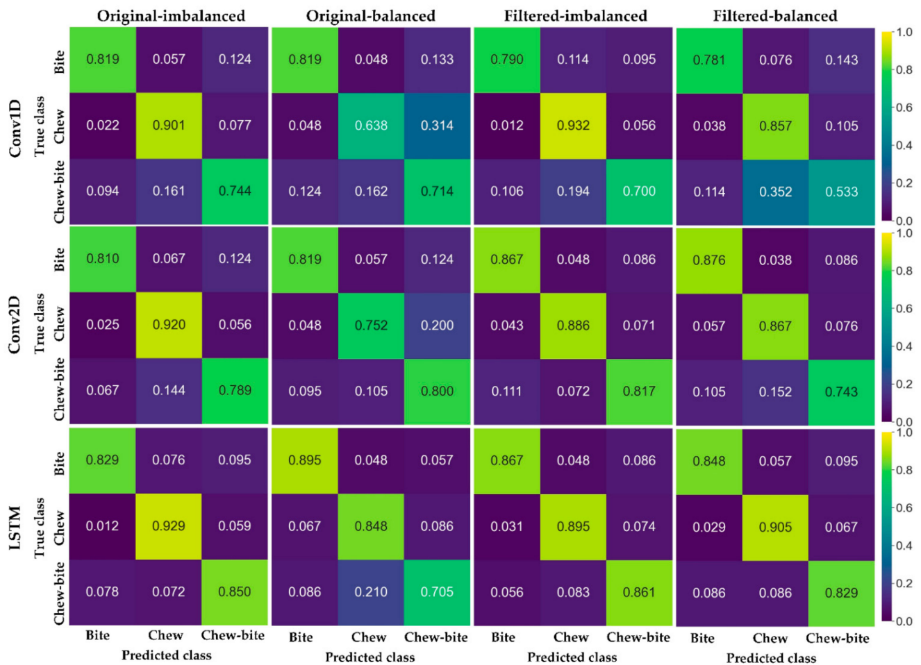
Figure 8. Confusion matrixes of the three deep learning models for classifying the ingestive behaviors in various datasets. Conv1D represents one-dimensional convolutional neural network; Conv2D represents two-dimensional convolutional neural network; and LSTM represents long short-term memory network. “Original” indicates the original dataset without any filtering; “Filtered” indicates the dataset was filtered with the bandstop filter to remove background beeping sounds; “imbalanced” indicates the dataset with unequal audio file sizes for the three ingestive behaviors; and “balanced” indicates the dataset with equal audio file sizes for the three ingestive behaviors.
