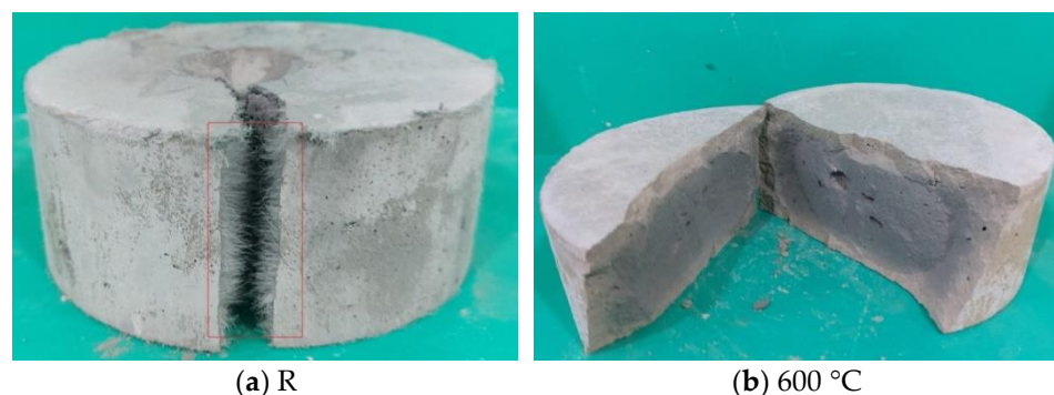
Figure 8. Physical appearance of PP fibers in the impact specimens before and after heating.
