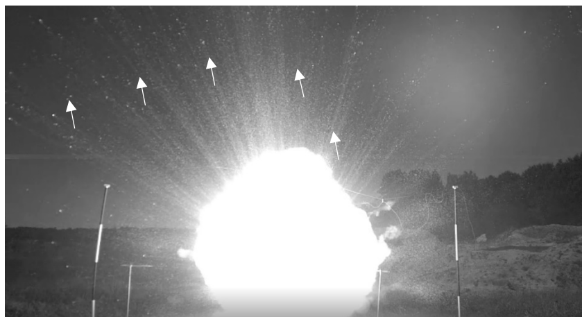
Figure 5. Image of the 500 g test (Test 7), in which burning Al particles (white arrows) were expelled.
