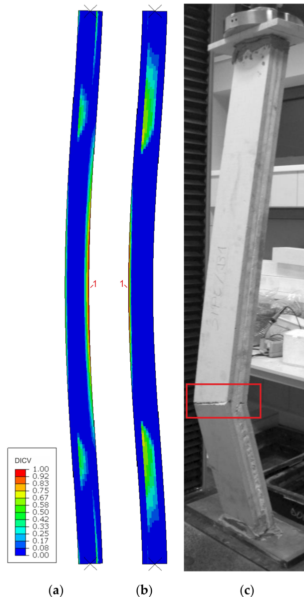
Figure 10. Comparison of failure modes in the L3 sample compression test obtained from FEA (a) MgO min, (b) MgO max variants, and (c) experimental observation.
