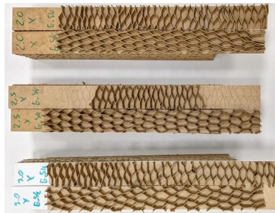
Figure 3. Examples of beams selected for testing.
