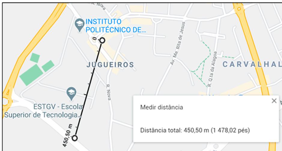
Figure 14. Distance calculation process for RSSI tests.
