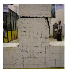
Figure 13. The failure mode of specimen BCJ3.
