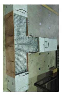
Figure 4. Wire mesh already installed on one side of the beam-column joint.
