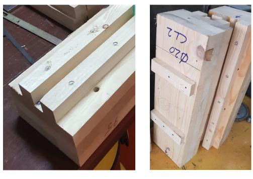
wooden beams that support the glass were 30 mm  $\times$  30 mm. The material and mechanical properties (acc. to [42,43]) of CL24h timber are shown in Tables 3 and 4.
