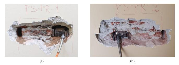
**Figure 18.** Masonry shear strength tests at measuring positions PS-PR-1 (**a**) and PS-PR-2 (**b**) on the ground floor (photo credit: L. Lulić).
