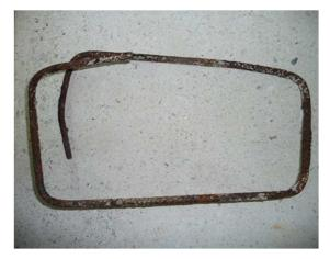
Figure 9. Removed corroded stirrup (position 8) with 65 days of exposure to induced deterioration.
