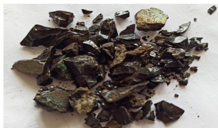
**Figure 1.** Production process for the PET bottle residual following constrained oxygen heating and residual condensation Method [37]: (a) waste plastic treatment reactor and (b) PET (EC number: 607-507-1) bottle residual before crushing.
