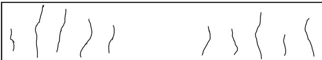
Figure 7. Cracking diagram for beam VCD-1 side A.
