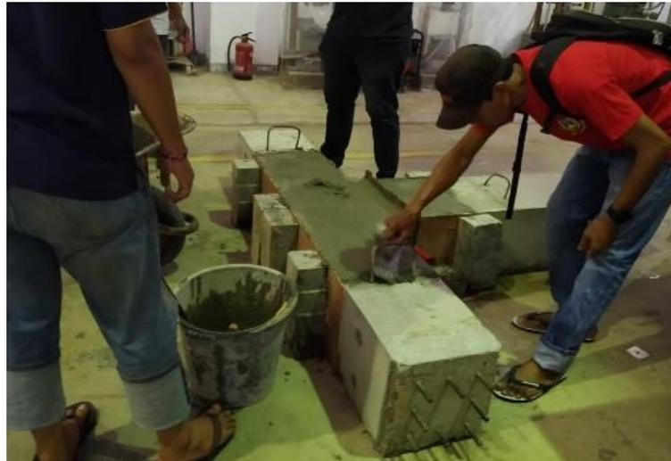
**Figure 5.** Re-casting the beam-column joint after installing the wire mesh.
