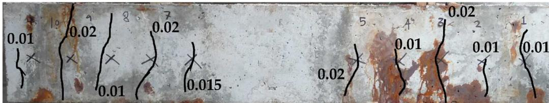
Figure 6. Visual appearance of beam VCD-1 side A after 65 days of applied deterioration; the crack widths are noted in cm.
