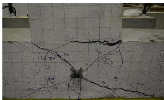
**Figure 9.** The failure mode of specimen BCJ1.
