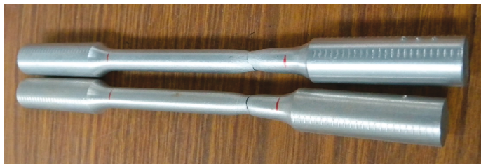
Figure 6. Tested A92030 tensile samples.
