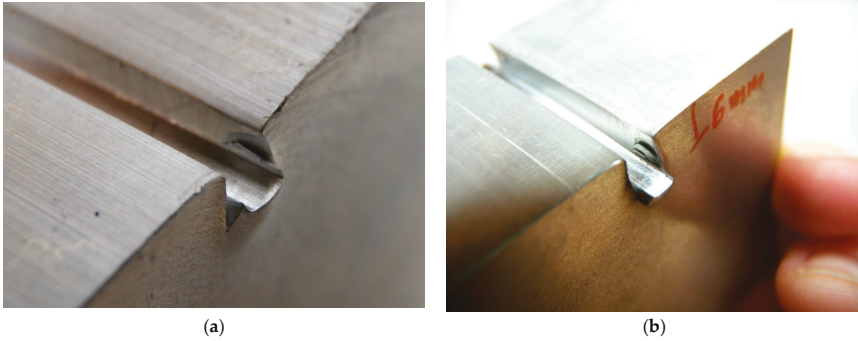
Figure 16. Cracks near the indenter boundary on specimen: E17 (a); and E23 (b) after indentation.
