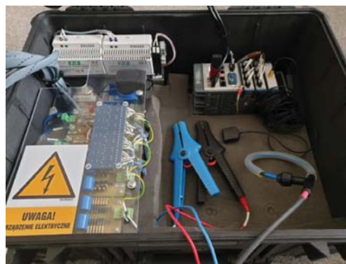
Figure 6. View of 1 MHz voltage and current recorder components.
