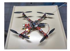
Figure 3. UAV equipped with the communication prototype.
