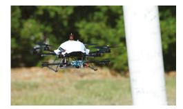
**Figure 1.** The vertical take-off and landing (VTOL) platform used for our pole inspection experiments. It includes a front-facing camera, downward-facing ultrasonic sensor and an onboard inertial measurement unit (IMU) for attitude control. All processing occurs onboard using a quad-core Acorn Risc Machine (ARM) Cortex-A9 processor.
