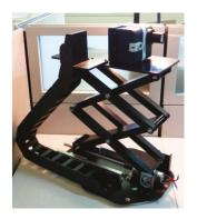
Figure 10. Completed scissor lift assembly with the 3D Flash LIDAR camera at the top.
