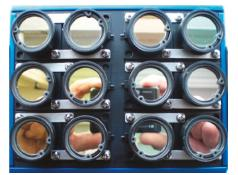
**Figure 3.** Tetracam Inc. miniature multi-camera array Mini-MCA 12 with mounted narrow-band (10–40 nm) filters that cover the spectral range between the visible and the near-infrared light (470–953 nm; both center wavelengths).
