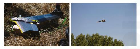
Figure 5. The eBee fixed-wing platform (left) and take-off phase (right).
