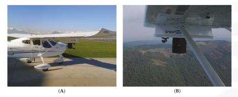
Figure 8. Sensor prototype mounted on the manned Digisky Tecnam P92 aircraft ready to take off (A) and during the flight (B).
