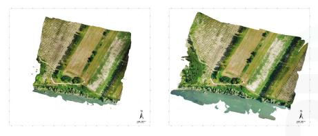
Figure 9. Orthophoto based on the images acquired with the multi-rotor UAV: 70-m flight height (left) and 150-m flight height (right).
