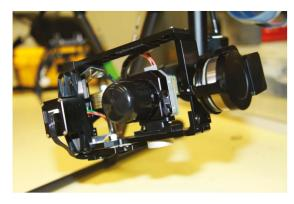
Figure 2. FLIR camera attached to the gimbal system.
