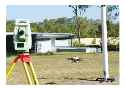
**Figure 19.** Experimental setup for outdoor flights. The VTOL platform is shown pointing towards the pole. An actuated surveying laser tracks a reflective beacon on the aircraft for position ground truth.
