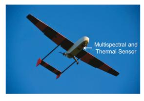
Figure 2. The Carolo P360 unmanned aerial vehicle (UAV) during a mission with open landing gear doors.
