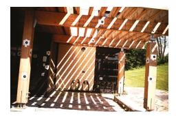
Figure 4. Test-field for platform calibration.
