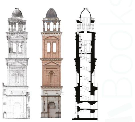
**Figure 11.** Santa Barbara bell tower. Laser scanning and photogrammetry data and a final elaboration of a vertical section obtained using both the technologies.
