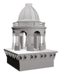
Figure 10. 3D model of the round temple for FEM analysis.
