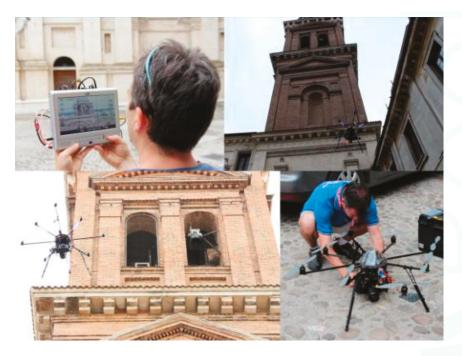
Figure 6. The octocopter employed for the bell tower acquisition, and the Wi-Fi camera controller.
