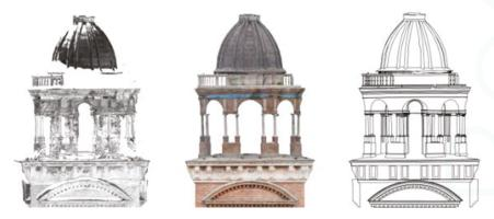
**Figure 9.** Comparison between the Santa Barbara bell tower's top laser scanner data and the respective surface orthophoto elaborated from the photogrammetric 3D model.
