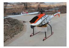
Figure 12. The unmanned helicopter and navigation sensor used for the flight tests.
