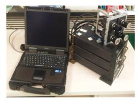
Figure 1. The four-camera multispectral mapping system.
