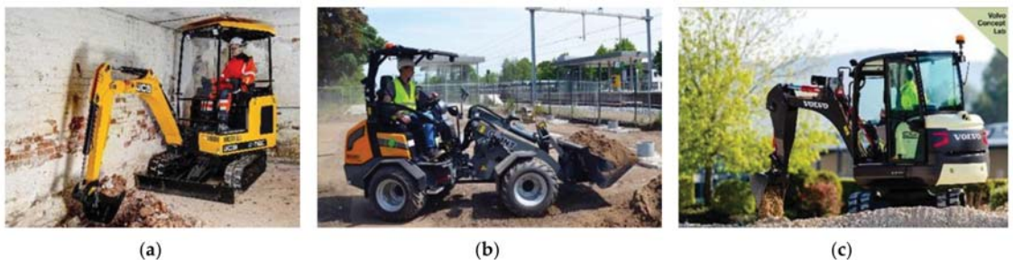
Figure 12. Electric construction vehicles. (a) JCB 19C-1E. (b) Tobroco-Giant E2200. (c) Volvo EX02. [98–100].
