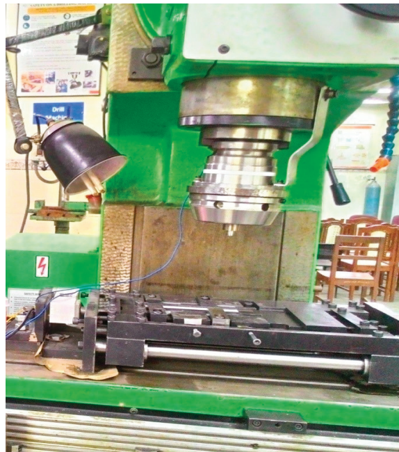
Figure 1. Experimental setup used for performing friction stir welding.
