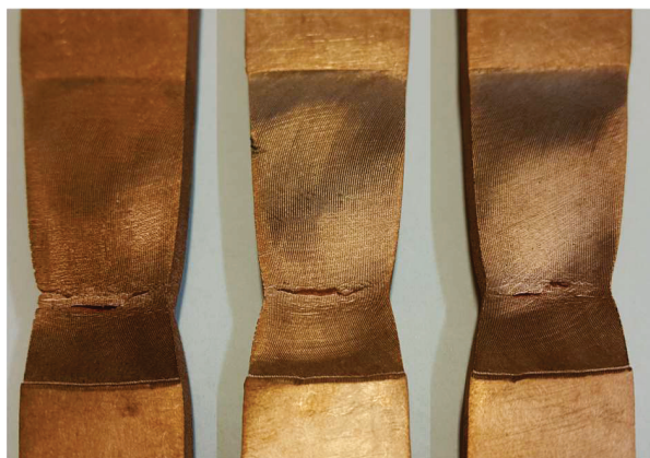
Figure 8. Fracture location of the tensile FSW joint samples.
