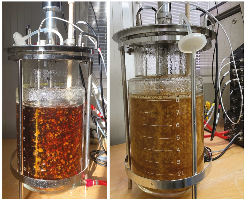
Figure 5. Different macroscopic growth patterns of the 15 day aged bioreactor cultures of I. obliquus mycelium grown in potato dextrose broth (left), showing extracellular pigment secretion and dispersed globular morphology, and optimized broth (right), unpigmented occupation of the entire bioreactor.
