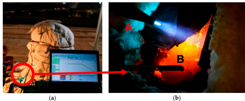
Figure 7. Welding process (a) the bell protected by fibro isolation; red circle—the place of welding (b) close-up of the place of welding. A—acetylene torch, B—bronze rod.
