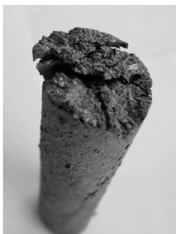
Figure 13. The sample without heat-treatment, one year after production—visible surface disintegration of structure.
