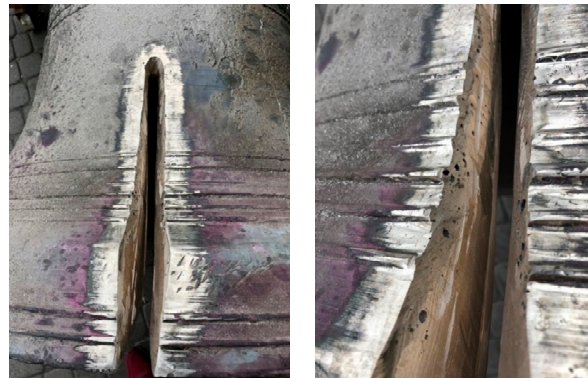
Figure 6. Mechanical treatment of the damaged place.
