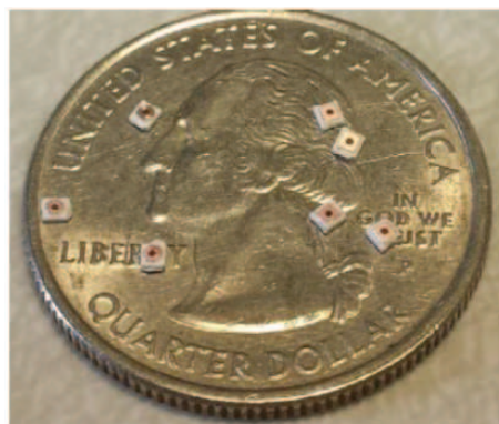
Figure 2. Manufactured measuring cups for the filling of magnetic particles in the MRS cavities.
