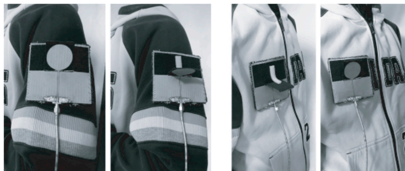
Figure 6. The measurement set-up for proposed fully textile reconfigurable UWB antenna with two monopole-like and a microstrip-like patterns ([89], reproduced courtesy of The Electromagnetics Academy).
