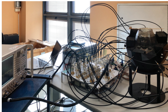
Figure 1. Overview of the realized 3D microwave imaging system prototype. From left to right: vector network analyzer (VNA), switching matrix and head phantom wearing a helmet interconnected to the switching matrix by means of coaxial cables.
