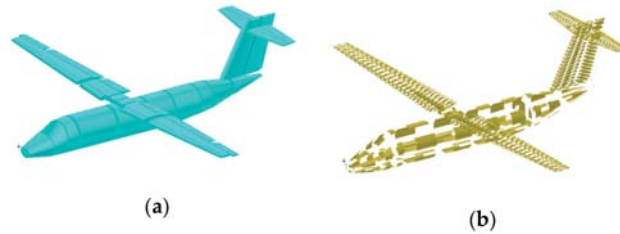
Figure 7. (a) Main sections of base configuration; (b) panels (details) of base configuration.
