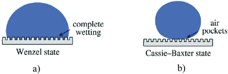
Figure 2. (a) Wenzel and (b) Cassie-Baxter models useful to describe the wetting of textured surfaces.
