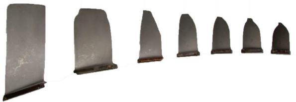
Figure 2. Erosive wear of compressor blades.
